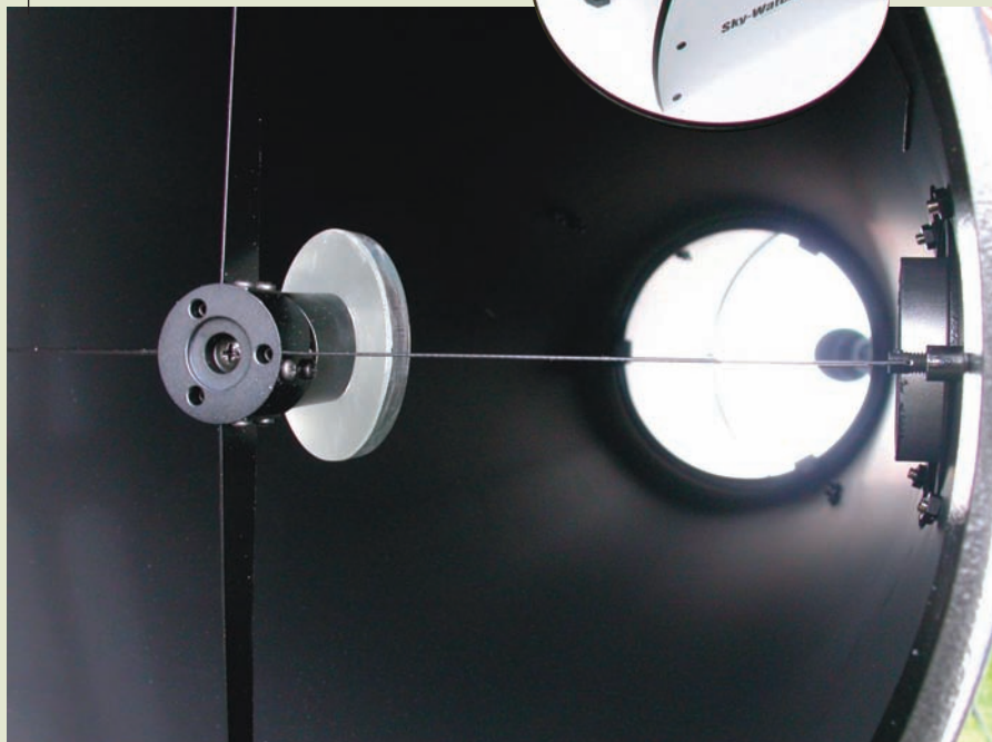
The secondary mirror in the foreground, and looking down the tube towards the primary mirror.
