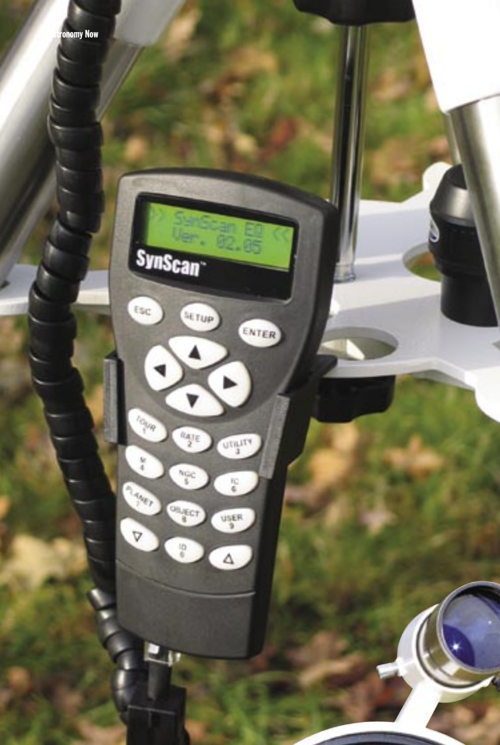
The SkyScan hand controller in a bracket attached to the eyepiece holder.
